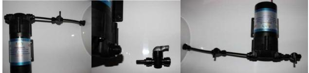
6. The above is an optional add-on if you wish to be able to close off your system to do any work on the pump without it leaking water when disconnected. This will require purchasing additional ball valves and union fittings. Contact us with any setup questions.
