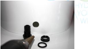
2. Take the ¼" bulkhead with plug and gasket, unscrew and remove bulkhead nut. Insert bulkhead through the hole you made from the inside of the reservoir. The gasket should be against the inside wall of the reservoir to make a water tight seal.
